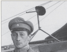
< Cabane strut, turnbuckle and wing warping control cable pulley A33 detail from a Fokker E.IV prototype (believed to be 122/15). Although the dark coloured cabane struts are not typical, the pulley and wing warping cable details are the same as for the E.II
