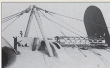
Cockpit coaming detail from Werner Notzke's FA 25 Fokker E.II. Note the ammunition feed chute G1 , cabane struts and style of IMG 08 'Spandau' cooling jacket P8 .
