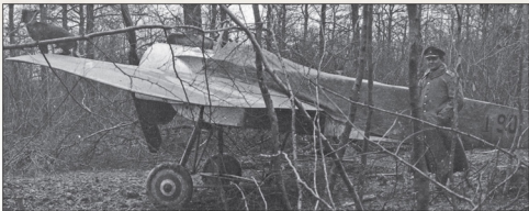
Fokker E.II 90/15 is shown here with protective coverings for the cockpit, IMG 08 'Spanau' and engine. Note the wheel markings, repainted serial number and dark/pale areas on the fuselage (possibly a very wide white eisernkreuz background). Additionally, a small dog is sitting on the wing tip.
