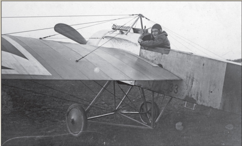
An unidentified pilot poses in Fokker E.II 33.15 B . Note the stained fuselage fabric, Germania propeller and how dark the wings appear compared to the fuselage fabric. Photos exist of a similarly marked Fokker E.II but the fuselage band spacing is not the same as that shown here and on pages 13 & 14.
