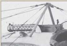
Cockpit coaming detail from Fokker E.II 33/15 A . Note the empty belt deflector A15 , fuel gauge A2 + 48 and style of IMG 08 'Spandau' cooling jacket P13 .
