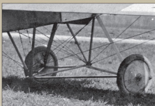
Undercarriage detail from D showing strut fairings and rigging details.
